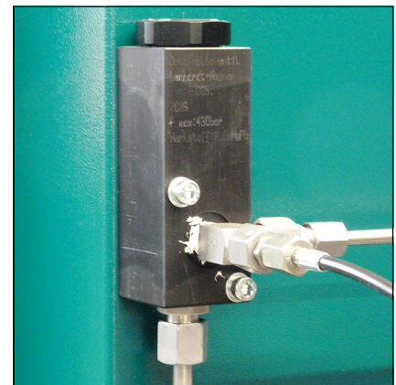
Pressure maintaining/non-return valve
