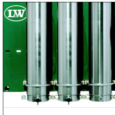
Fig. 3 - Loosen u-clamps and pipe connections
