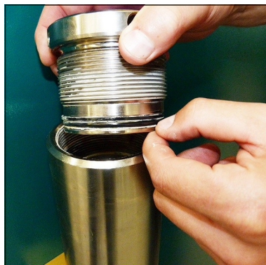
Fig. 2 - Change o-ring and back-up rings
