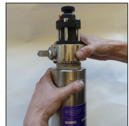
Fig. 3 - Open filter cover
