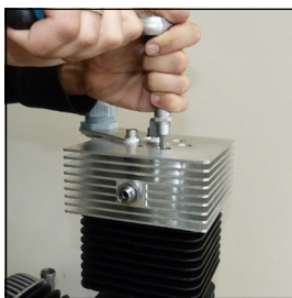
Fig. 1 - Loose valve head screws
