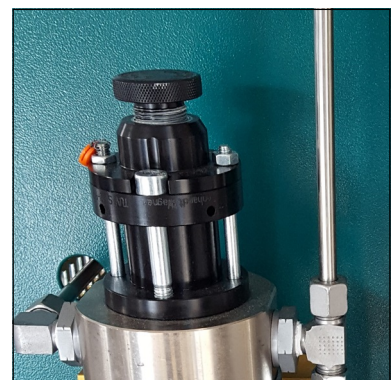
Safety valve 4th stage
