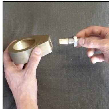
Abb. 8 - Change sinter filter
