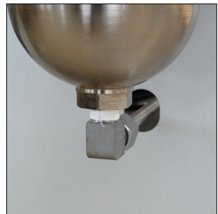
Fig. 2 - Loosen pipes and nuts
