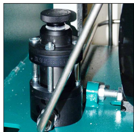
Safety valve 4th stage
