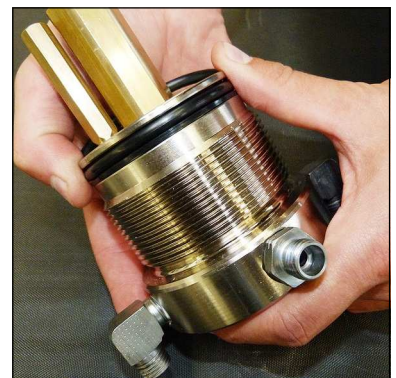
Fig. 4 - Change o-ring and back-up rings
