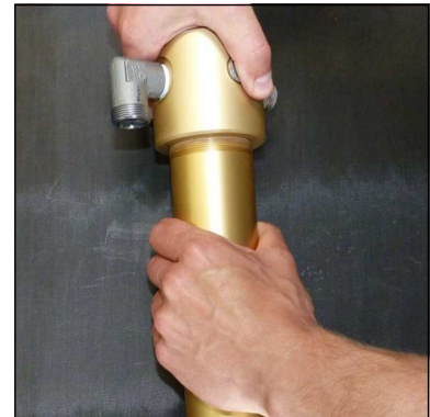
Fig. 1 - Unscrew and remove filter top
