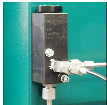
Pressure maintaining/non-return valve
