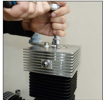
Fig. 1 - Loosen valve head screws
