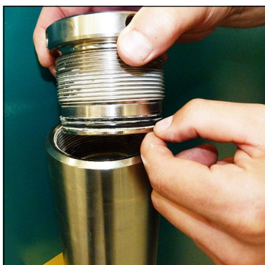
Fig. 2 - Change o-ring and back-up rings
