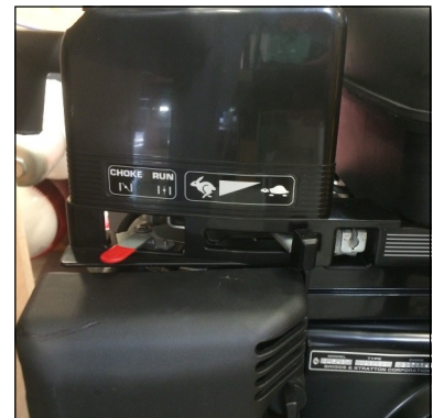
Fig. 1 - Fuel valve and speed control
