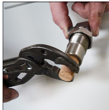
Fig. 3 - Change sinter filter
