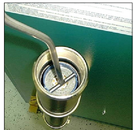
Fig. 2 - Place the T-piece end of the filter key in the top of the filter cartridge.
