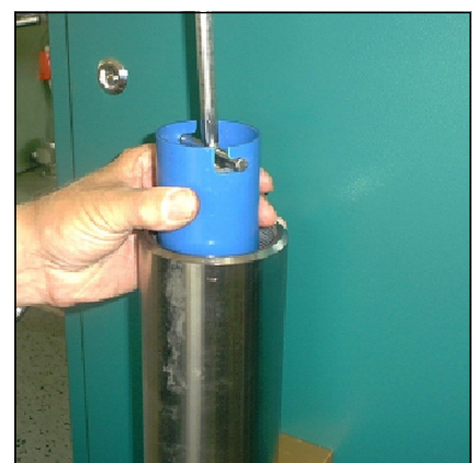
Fig. 3 - Pull the cartridge out of the housing.
