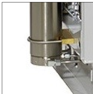
Fig. 3 - Loosen pipe connections and nuts
