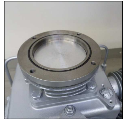
Fig. 1 - Change lower gasket (o-ring)
