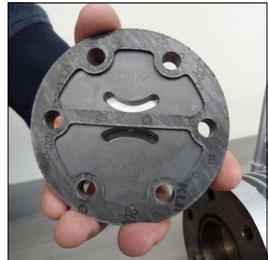
Fig. 2 - Correct mounting position of upper valve gasket
