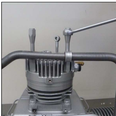
Fig. 5 - Remove cooling pipe bracket
