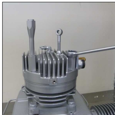
Fig. 6 - Remove special hexagon bolt
