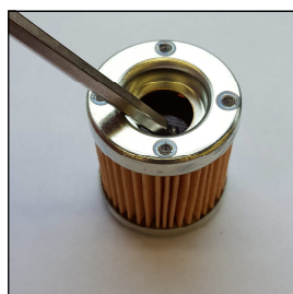
View bypass valve
