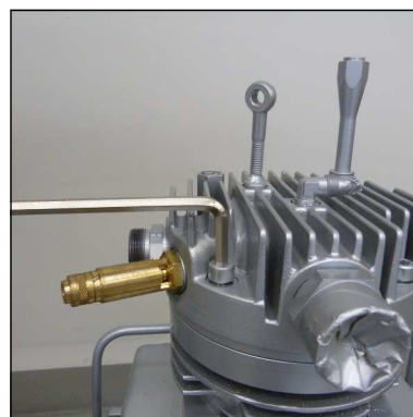
Fig. 4 - Tighten mounting screws
