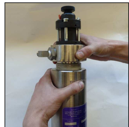
Fig. 3 - Open pre-filter cover
