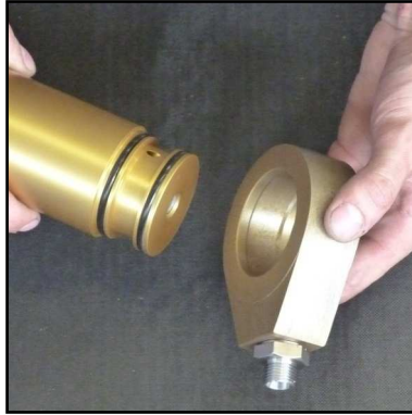
Abb. 5 - Remove the base ring
