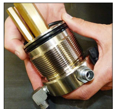
Fig. 4 - Change o-ring and back-up rings
