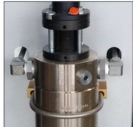
Fig. 1 - Loosen pipe connections and mounting screws
