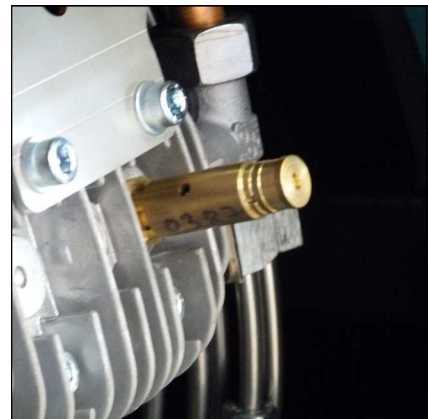
Safety valve 2nd stage
