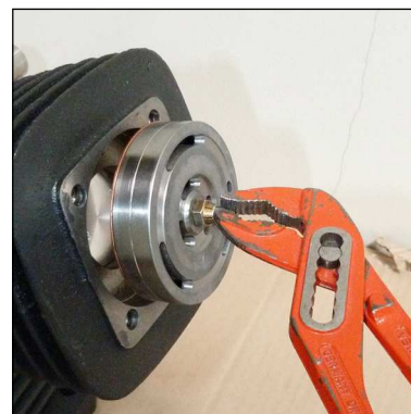
Fig. 2 - Pull out inlet and outlet valve
