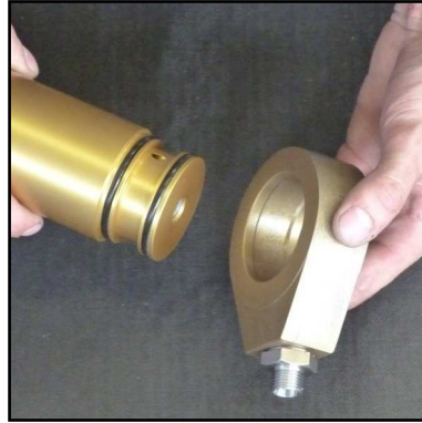
Abb. 5 - Remove the base ring
