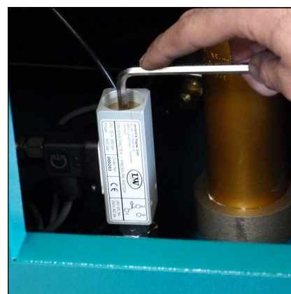
Final pressure switch
