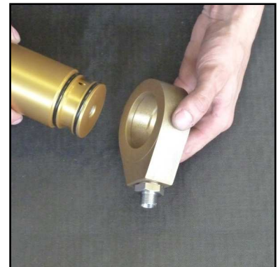
Abb. 6 - Remove the base ring
