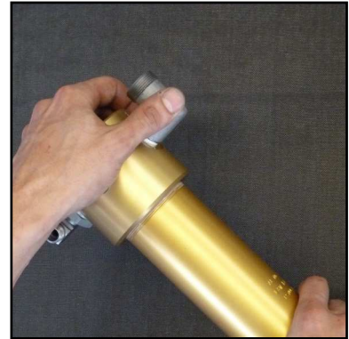
Fig. 1 - Unscrew and remove filter top
