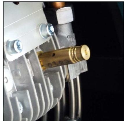
Safety valve 2nd stage
