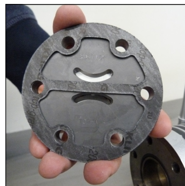
Fig. 2 - Correct mounting position of upper valve gasket
