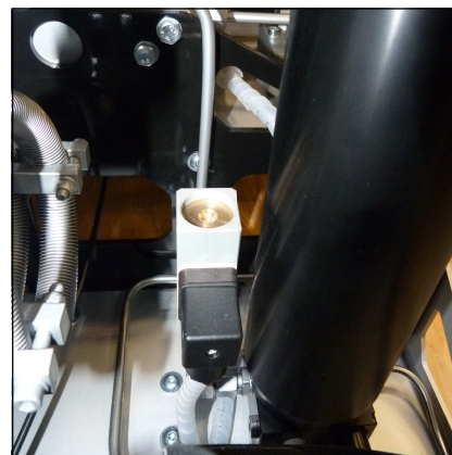
Final pressure switch
