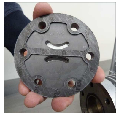
Fig. 2 - Correct mounting position of upper valve gasket
