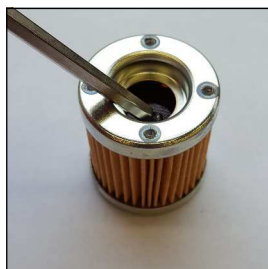
View bypass valve
