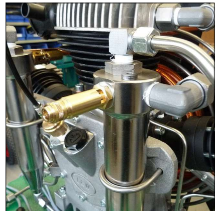
Safety valve 1st stage
