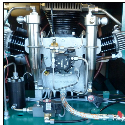
Fig. 1 Oil / water separators 1st and 2nd stage with automatic condensate drain system
