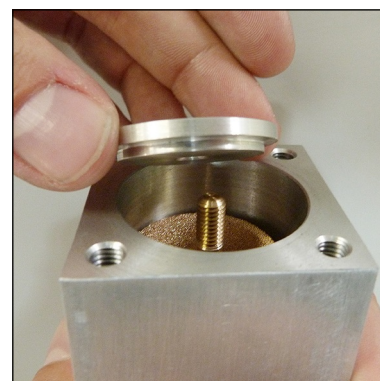
Fig. 5 - Place filter washer and washer
