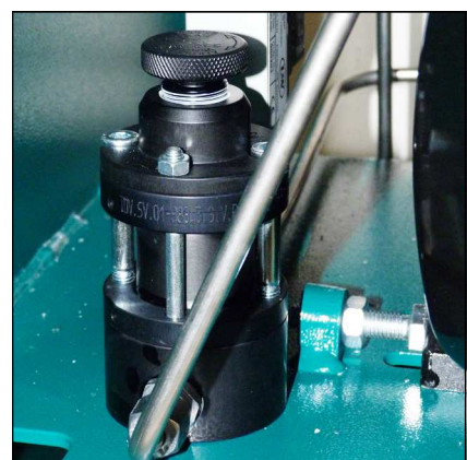
Safety valve 3rd stage
