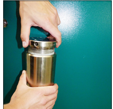
Fig. 1 - Open Filter cover
