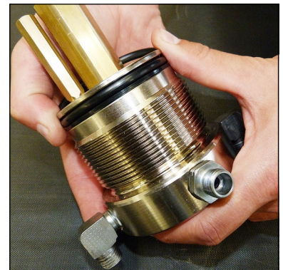
Fig. 4 - Change o-ring and back-up rings
