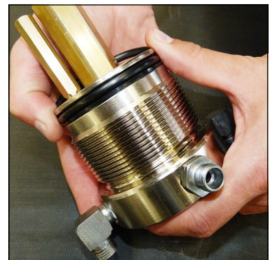
Fig. 4 - Change o-ring and back-up rings
