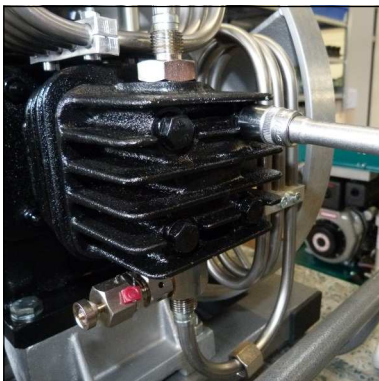
Fig. 2 - Loosen valve head screws
