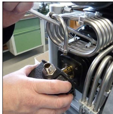
Fig. 3 - Remove valve head
