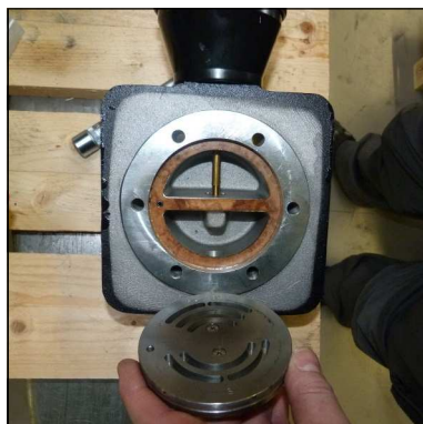
Fig. 2 - Correct position of in-and outlet valve
