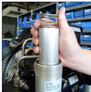
Abb. 2 - Remove filter cartridge
