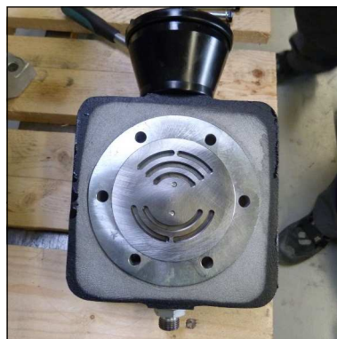
Fig. 3 - Correct position of in-and outlet valve
