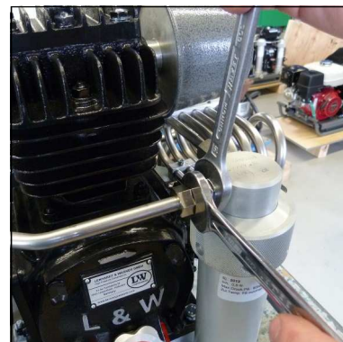
Fig. 1 - Loosen pipe connections of the water separator
