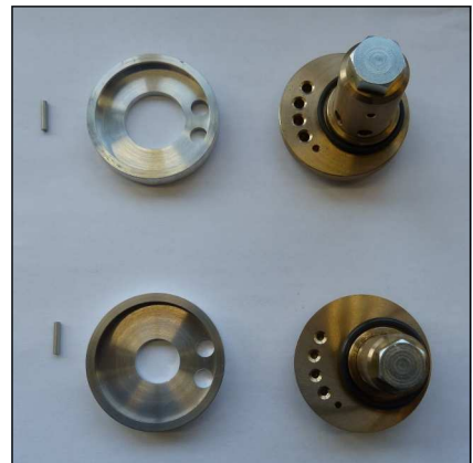
Fig. 2 - In - and outlet valve c/w gaskets 2nd stage (top) und 3. Stufe (below)
