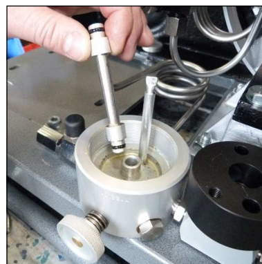
Abb. 5 - Remove duct collar and change o-rings
