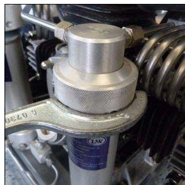
Abb. 5 - Tighten lock ring
