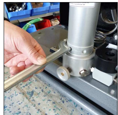
Abb. 3 - Turn off filter housing
