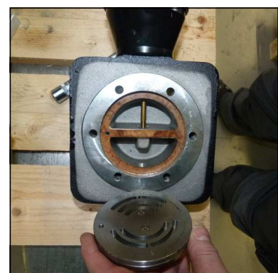
Fig. 5 - Remove in- and outlet valve
