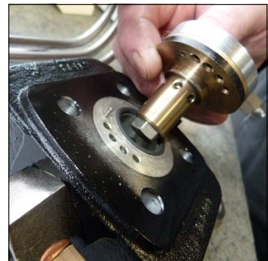
Fig. 4 - Ensure correct valve position (centre pin)
