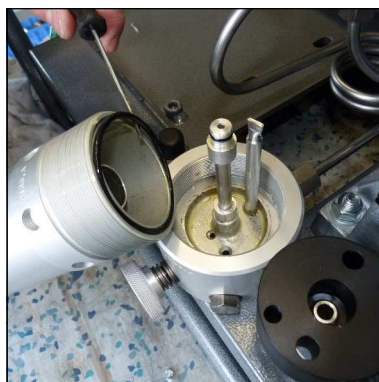
Abb. 4 - Remove lock ring
