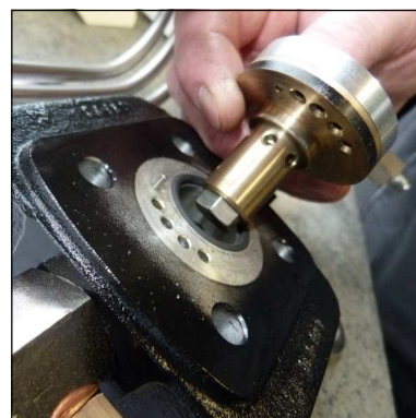
Fig. 5 - Ensure correct valve position (centre pin)
