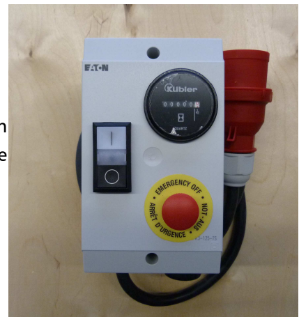
Remote control box c/w hour counter
