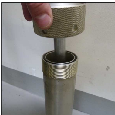
Abb. 4 - Remove lock ring and change o-ring
