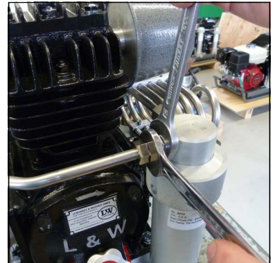
Fig. 1 - Loosen pipe connections of the water separator
