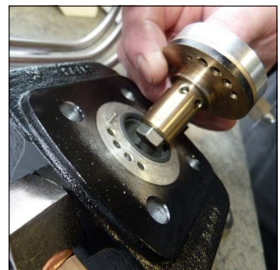
Fig. 4 - Ensure correct valve position (centre pin)
