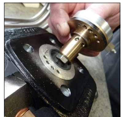
Fig. 5 - Ensure correct valve position (centre pin)
