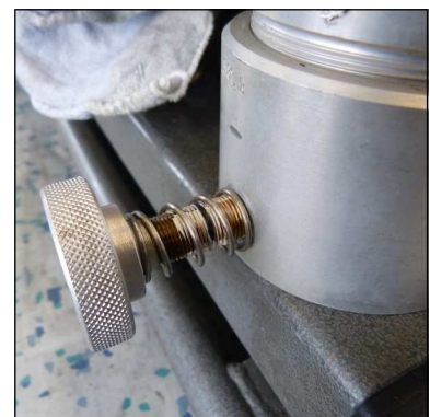
Abb. 6 - O-ring, condensate drain valve
