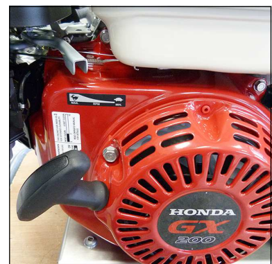
Fig. 2 - Speed control and pull start
