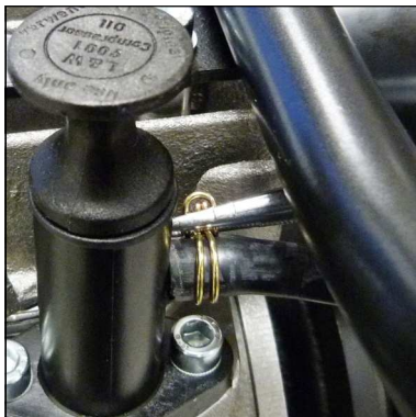
Fig. 2 - Remove spring wire clamp
