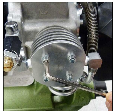
Fig. 2 - Loosen valve head screws
