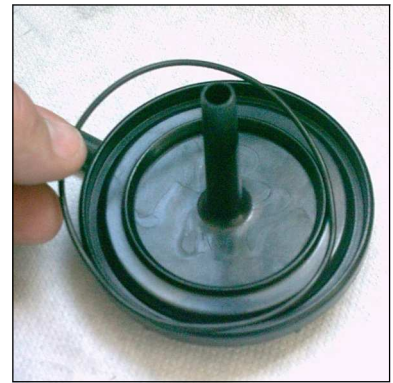
Fig. 3 - Place o-ring into the filter housing
