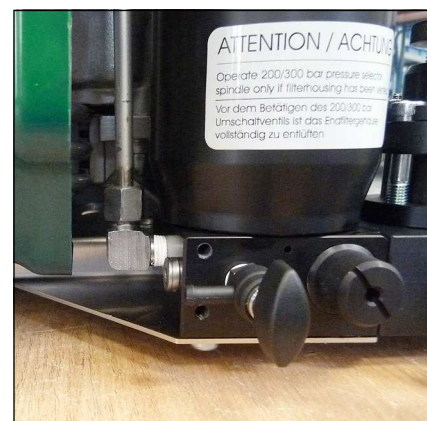
Fig. 2 - Condensate drain valve 3.stage
