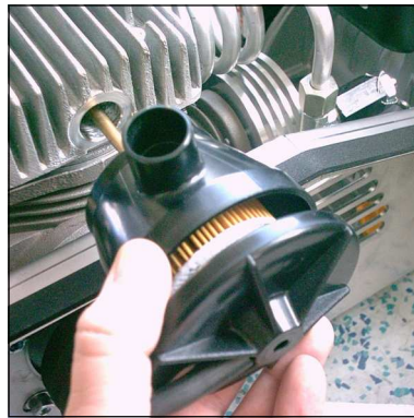
Fig. 2 - Pull out filter housing carefully
