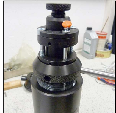
Fig. 1 - Remove/screw in filter cover
