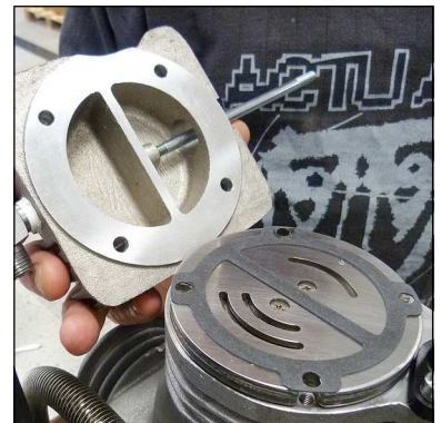
Fig. 4 - Remove valve head
