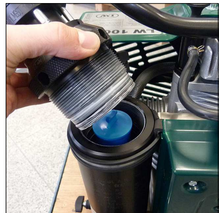
Fig. 2 - Remove filter housing cover
