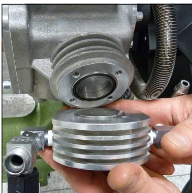
Fig. 3 - Remove valve head with inlet and outlet valve
