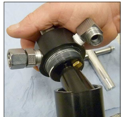
Fig. 3 - Turn off and remove separator head
