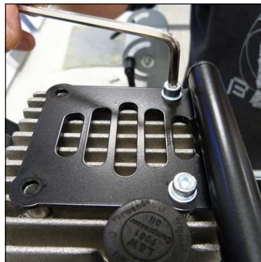
Fig. 3 - Loosen valve head screws
