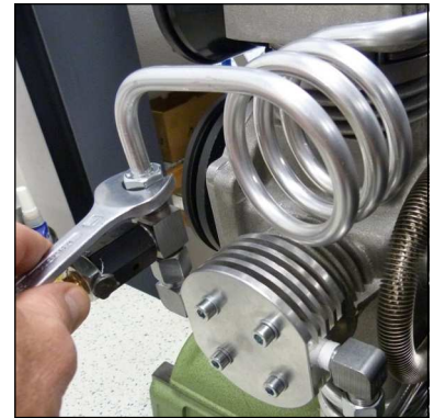
Fig. 1 - Loosen pipe connections
