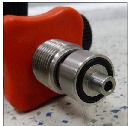
Fig. 1 - O-ring at the filling valve
