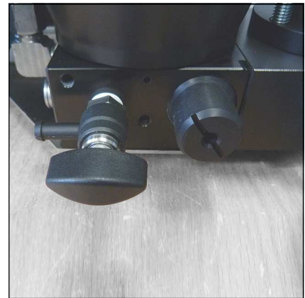
Drain valve and pressure maintaining / non return valve
