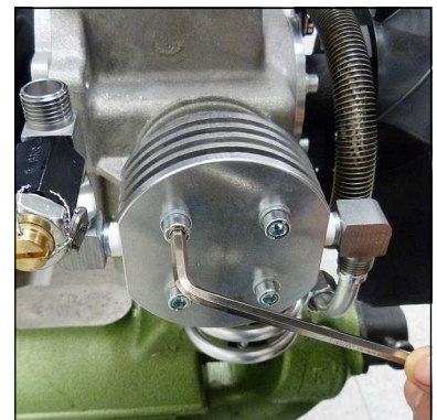
Fig. 2 - Loosen valve head screws
