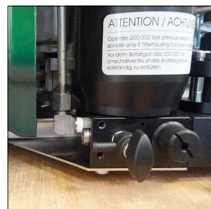
Fig. 2 - Condensate drain valve 3.stage
