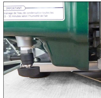
Fig. 1 - Condensate drain valve 1.stage
