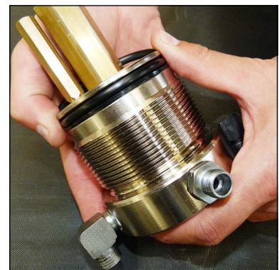
Fig. 4 - Change o-ring and back-up rings
