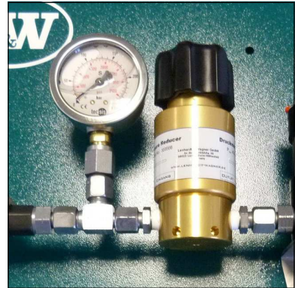
Fig. 1 - Inlet pressure gauge
